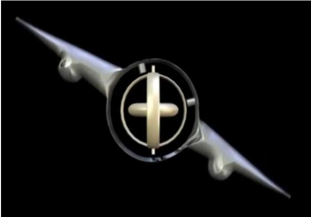
89. Plane tilted, gyroscope compensates
